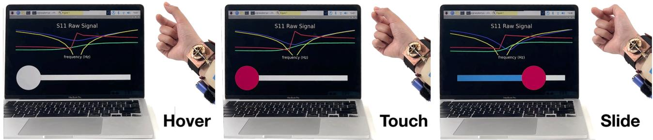
**Figure 11:** In this micro-gesture example sequence, a user can use their thumb and index finger like a slider. Laptop included to illustrate the captured signal and slider state.
