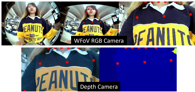
Figure 6. Result of the fusion of WFoV RGB and NFoV depth cameras. The red dots on the images are body keypoints. The upper three images are from the WFoV camera and the lower two from the depth camera.
