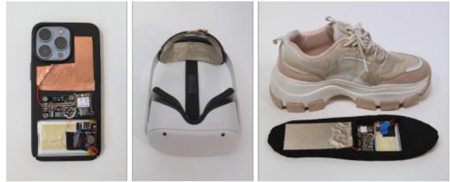
Figure 5: In addition to a basic velcro strap (seen in Figure 14), we created three prototype transmitters built into existing objects: phone, XR headset, and shoes.
