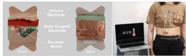
Figure 14: Patches for longitudinal biometric monitoring could benefit from Power-over-Skin. As a proof of concept, we built a body temperature monitor that logs readings roughly every five minutes over Bluetooth.
