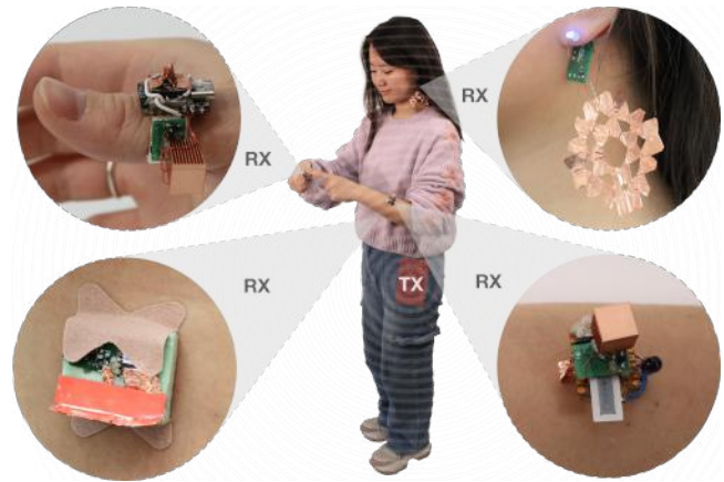
Figure 1: Power-over-Skin allows a single worn transmitter (e.g., stored in a pocket) to provide power to a constellation of small, worn, battery-free devices. Example devices we created include (clockwise from top-left): a controller ring that sends user input over BLE, earrings that blink, a sun exposure monitor with an e-ink display, and body temperature patch that logs data every five minutes.
