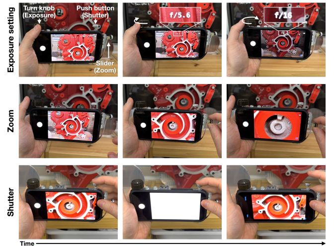
Figure 7: One of two example interactive phone cases we made (see also Figure 9). Here, a camera-enthusiast case provides mechanical controls for exposure, zoom, and shutter. See Figure 13 for close-ups of example widget designs.
